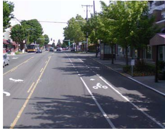
Figure MR-2.2: A bicycle path as part of the roadway (image from Google Maps).
