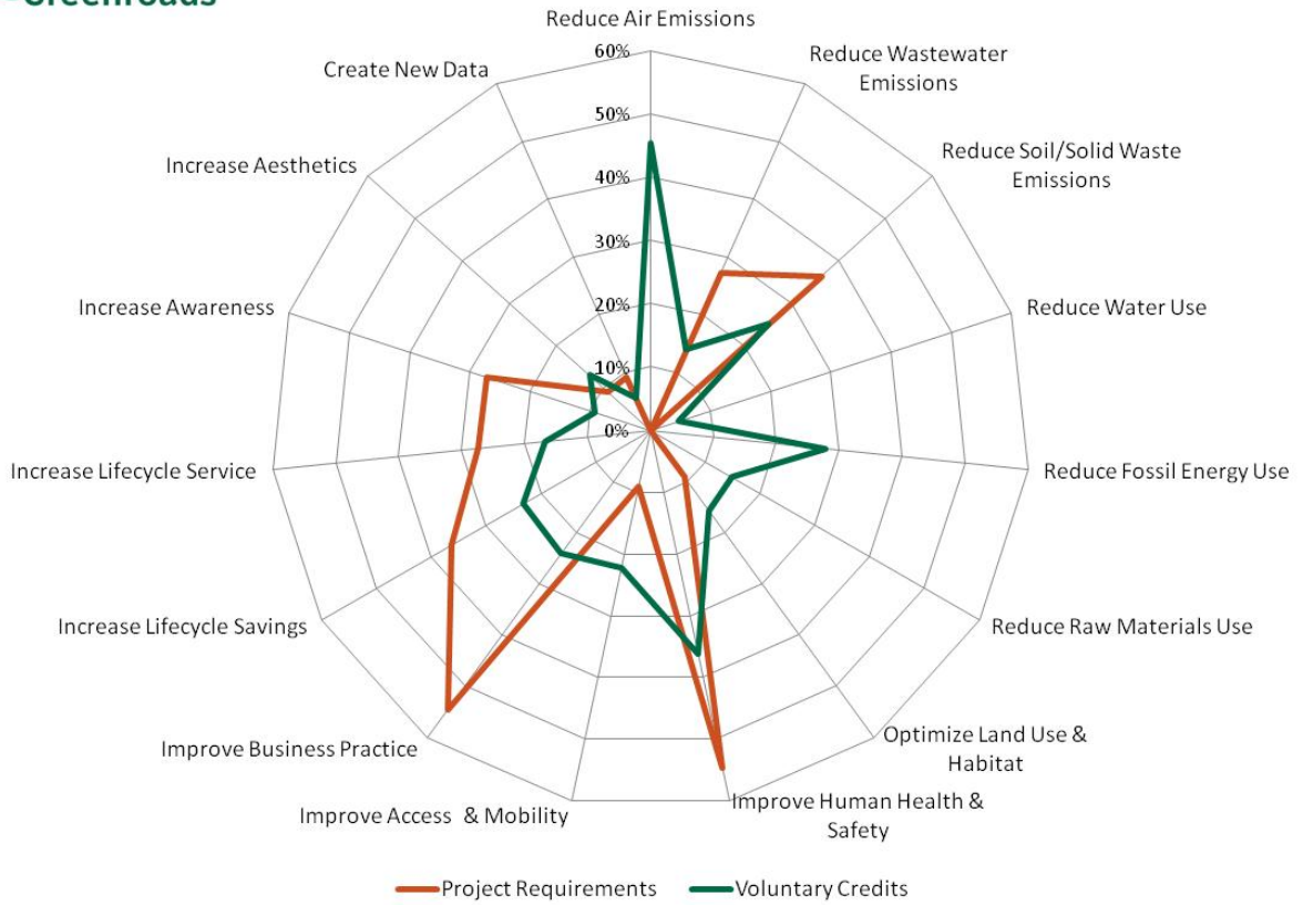
Figure 1.3: Spider graph showing the percentage of Project Requirements and Voluntary Credit points (not including any Custom Credits) that can be traced to one of sixteen sustainability benefits as defined by Greenroads. Note that “create energy” has been excluded because no credits do this currently.
